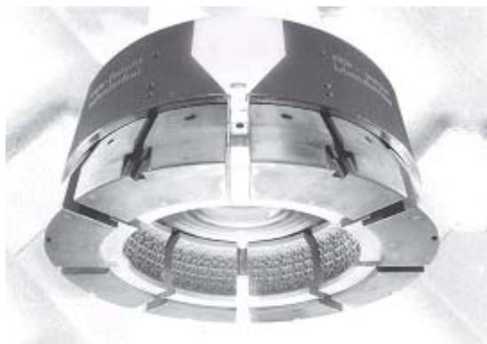
Lubrication is applied to top, bottom, and sides of mold.
